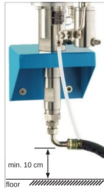
Fig. 20 Mounting the wall bracket
