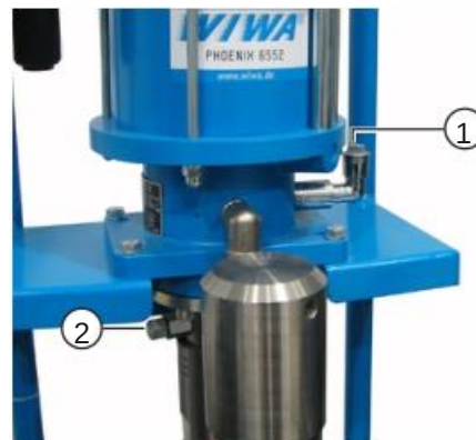
Fig. 31 Filling in (1) and draining (2) release agent for PHOENIX
